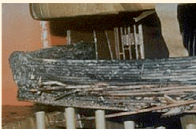
Figure 3. Burnt-out transformer from an electrical power distribution network caused by the March 1989 flare.
